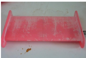
Rough blade: P120 sandpaper (125 µm particle diameter)
