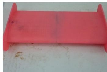
Smooth blade: P4000 sandpaper (6 µm particle diameter)
